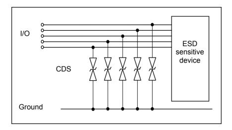
Protection of I/O Lines with discrete CeraDiodes
