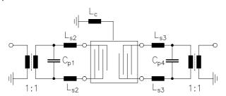
$$\begin{array}{lll} L_c & = 39 \text{ nH} \\ C_{p1} & = C_{p4} = 6.8 \text{ pF} \\ L_{s2} & = L_{s3} = 33 \text{ nH} \end{array}$$
