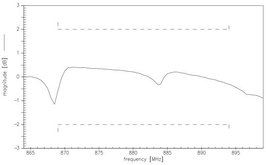
Input phase balance ( $\phi(S_{31})-\phi(S_{21})+180^{\circ}$ ; measurement)
