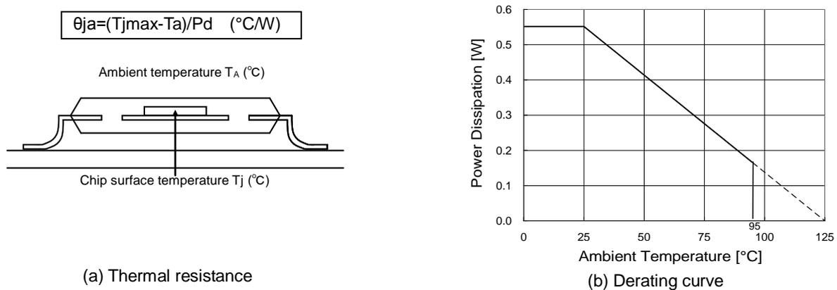
Figure 13. Thermal resistance and derating curve
