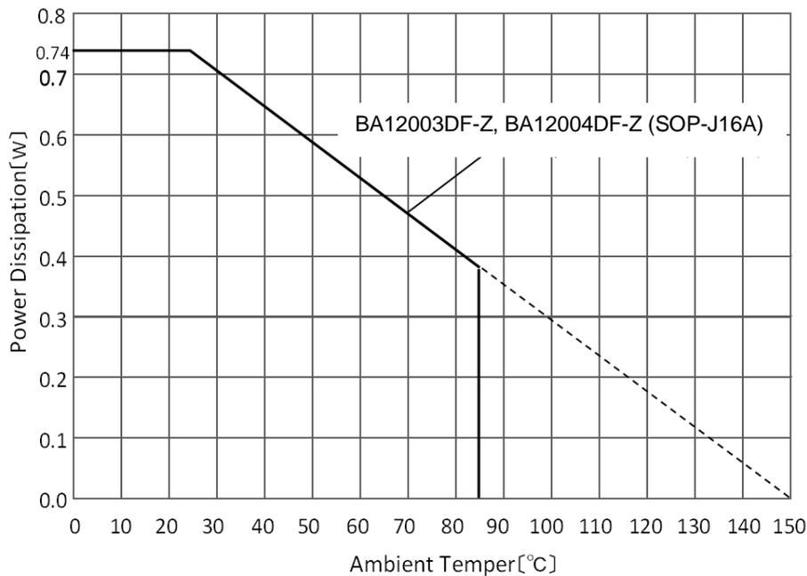
Figure 14. Derating curve
