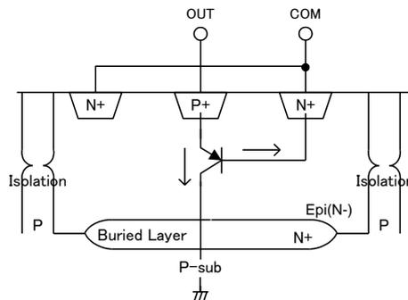
Figure 16. Construction of output clamp diode
