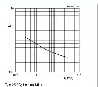
Figure 2. Diode forward resistance as a function of forward current (typical values)
