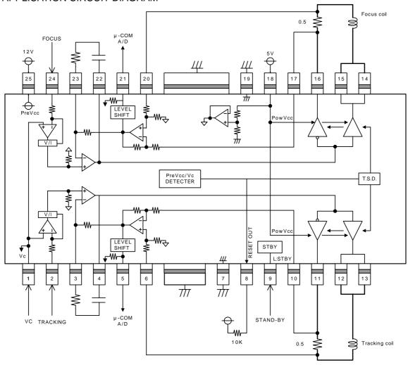
T.S.D: (Thermal shutdown) Resistance unit:  $[\Omega]$
