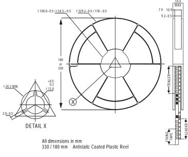
NOTES: 8mm Tape 8mm Tape Size of Reel 330 mm (13") 180 mm (7")
