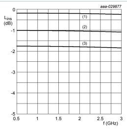
Diode inserted in series with a 50  $\Omega$  strip line circuit and biased via the analyzer T-network. T<sub>amb</sub> = 25 °C.
