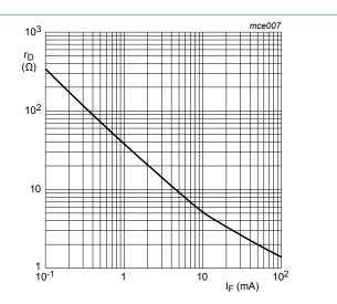
$f = 100 \text{ MHz}; T_j = 25 ^{\circ}\text{C}$
