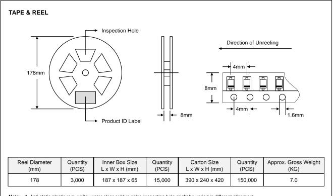
Note: 1. Anti-static plastic reel, white, water clear or blue color. Inspection hole might be varied in different alignment. 2. Components are packed in accordance with EIA standard 481-1 and 481-2.
