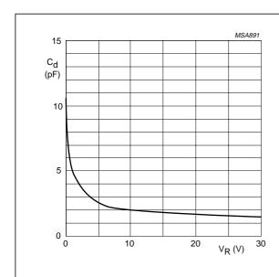
f = 1 MHz;  $T_{amb} = 25 \, ^{\circ}\text{C}$ .
