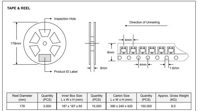
Note: 1. Anti-static plastic reel, white, water clear or blue color. Inspection hole might be varied in different alignment. 2. Components are packed in accordance with EIA standard 481-1 and 481-2.
