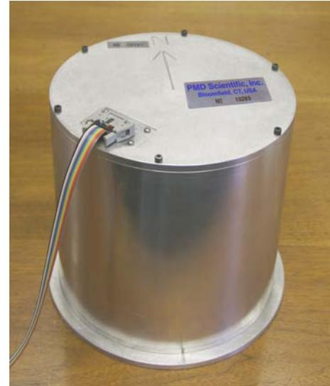
level and is used for strong motion applications. Both versions have the same dynamic range, which is shifted up by approximately 10db in the '*SM*' relatively to the standard '*LN*' version. The **BB313** instruments have been recently redesigned. Also available are a single component version **BB313U**, a very low power customized lightweight, compact ocean-bottom seismometer (OBS) **BB313-OBS** (photo on the right above), and a narrow (83mm diameter) borehole model **BB313-BH**
