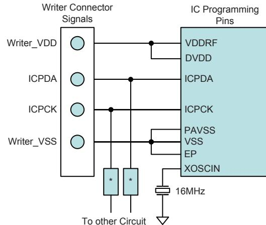
Note: \* may be resistor or capacitor - the resistance of \* must be greater than 1kΩ and the capacitance of \* must be less than 1nF.
