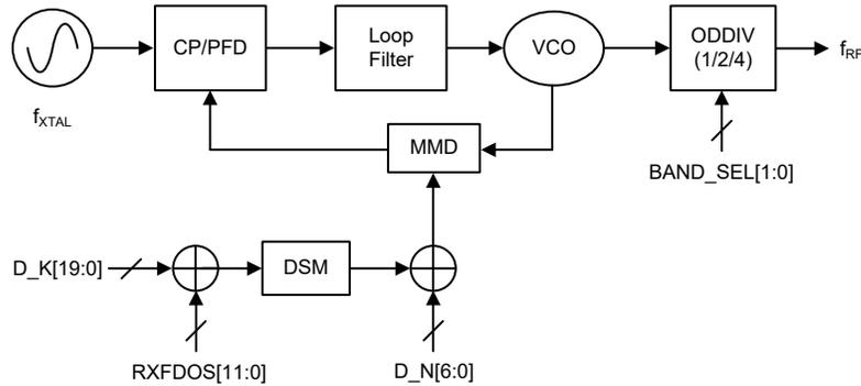
The RF transceiver frequency is generated by a high resolution fractional-N Delta Sigma frequency synthesizer. By appropriate setting on the configuration parameters D\_N[6:0] and D\_K[19:0], a low-noise LO frequency can be generated to comply with various radio regulatory standards including ETSI EN, FCC, etc.
