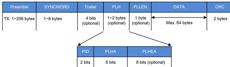
The slave side in the auto-ack mode uses the packet format as the following to be an acknowledge packet transmitted to master. Note that there is no payload data field used in the acknowledge packet.
