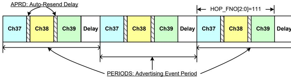
**PKT\_APRD[4:0]:** Packet format auto-resend delay, 250µs (Min.) ~ 8ms (Max.)
