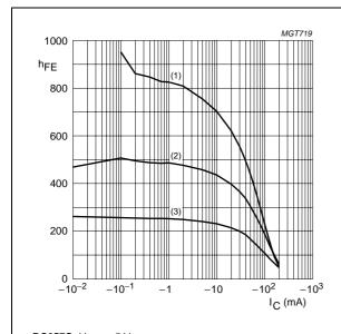
**BC857C;**  $V_{CE} = -5 \text{ V}.$
