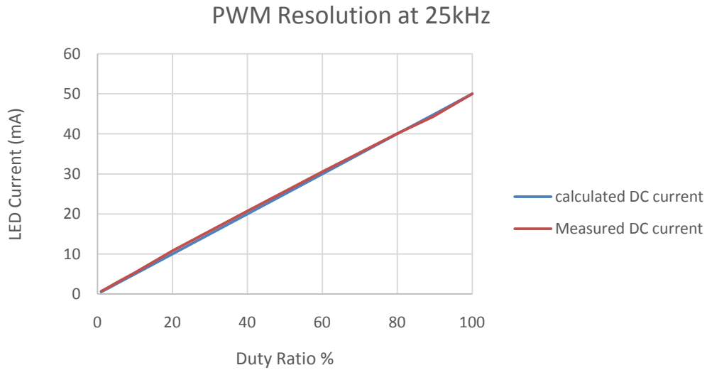
Figure 8 PWM Resolution with Power Path Switching (Refer to Figure 3c)
