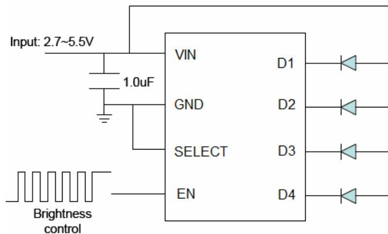
Figure 1: Application Circuit for Co-Anode Connection.
