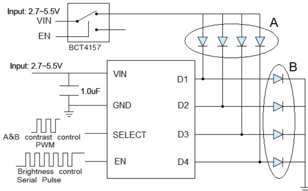
Figure 3: Application Circuit for Co-Anode & Co-Cathode Connection.
