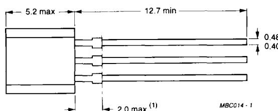
Note (1) Terminal dimensions within this zone are uncontrolled to allow for flow of plastic and terminal irregularities.
