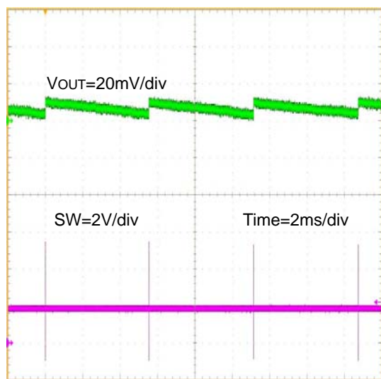
Figure 30. Output Ripple ( V_{IN} = 5V , V_{OUT} = 1.8V , I_{OUT} = 0A )
