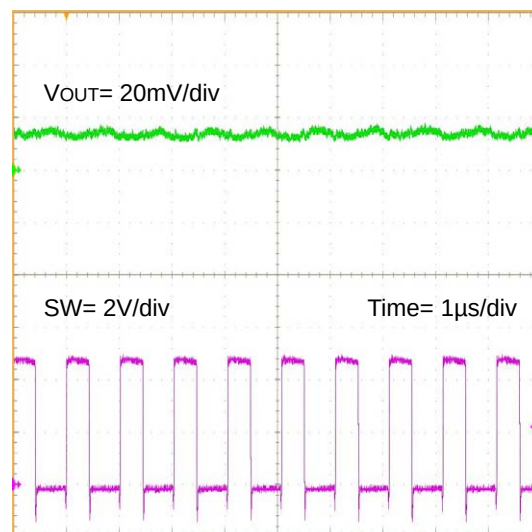
Figure 31. Output Ripple ( V_{IN}= 5V , V_{OUT}= 1.8V , I_{OUT}= 6A )
