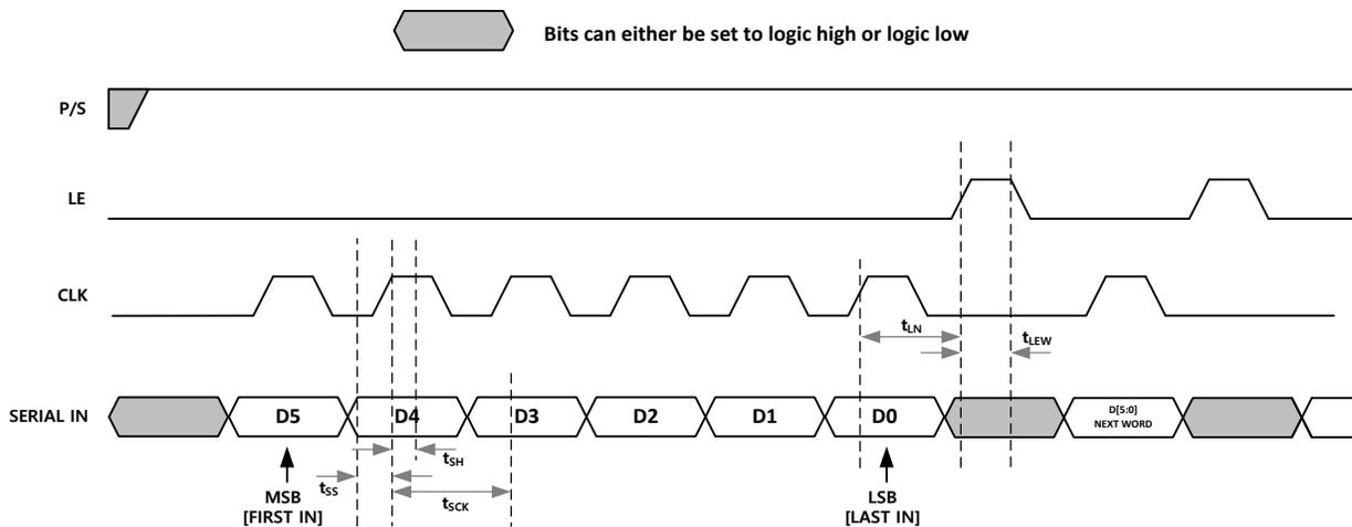
The BDA4620 has a 3-wire serial peripheral interface (SPI): serial data input (SERIN), clock (CLK), and latch enable (LE). The serial control interface is activated when P/S is set to HIGH.
