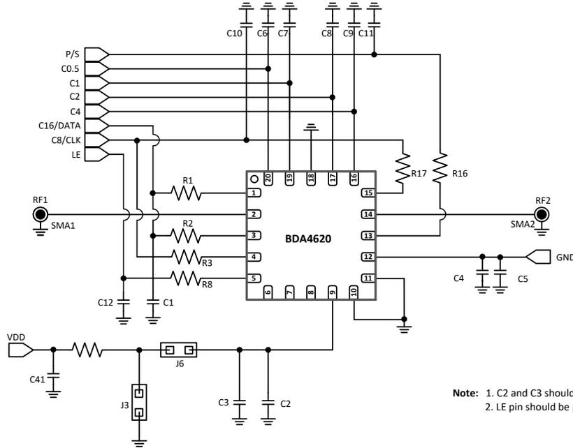
Note: 1. C2 and C3 should be placed near the device.
