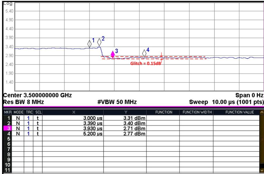
Figure 33. Attenuation Transient (16 to 15.5dB, Pin=18dBm)
