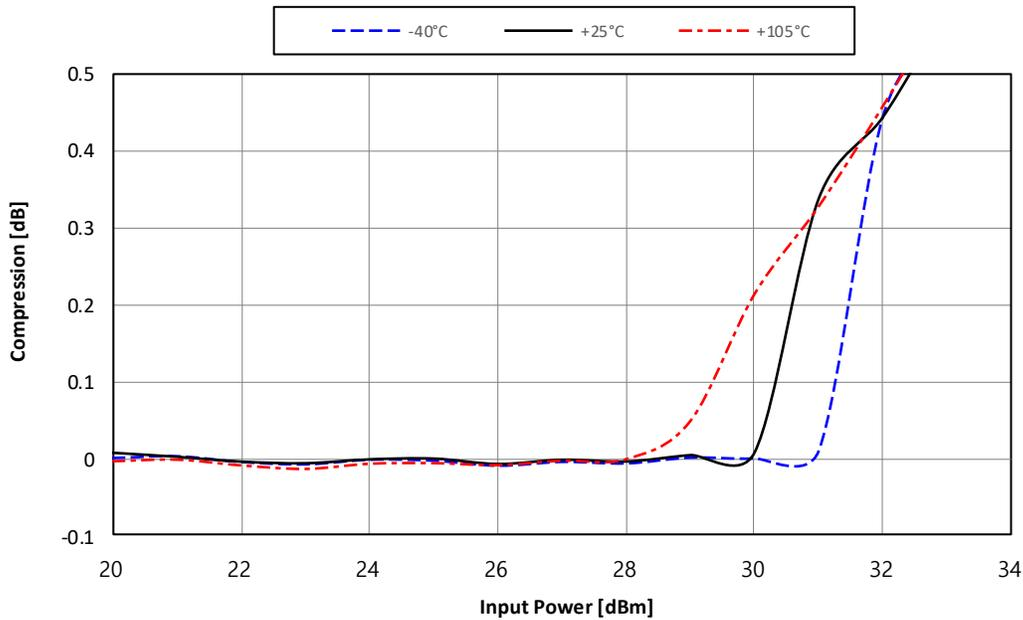
Figure 27. Input 0.1dB Compression @4500MHz vs Temperature
