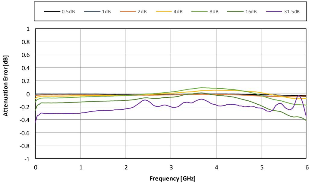
Figure 31. 0.5dB Step Attenuation Error vs Frequency
