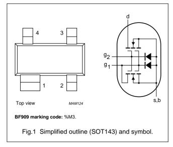
transistor consists of an amplifier MOS-FET with source and substrate interconnected and an internal bias circuit to ensure good cross-modulation performance during AGC.
