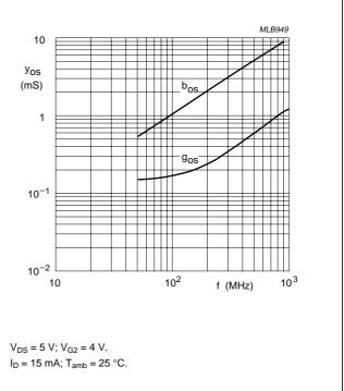
Fig.17 Output admittance as a function of frequency; typical values.
