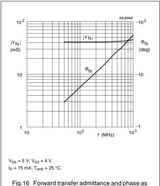
Fig.16 Forward transfer admittance and phase as a function of frequency; typical values.
