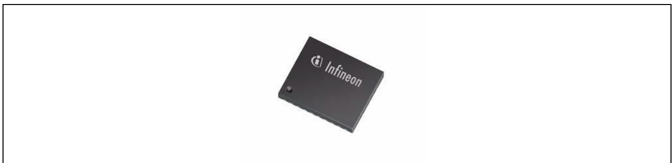
Figure 1 BGSF1717MN26 package in TSNP-26-3
