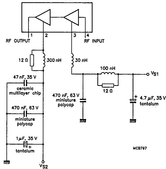
Fig.4 Decoupling arrangement.
