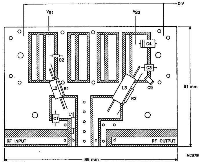
Epoxy fibre-glass board, 1/16 inch thick,  $\epsilon_r = 4.5$ .
