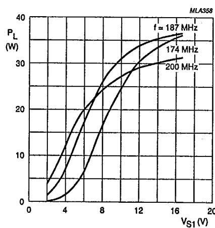
$P_D = 300 \text{ mW}; V_{S2} = 12.5 \text{ V.}$
