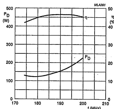
$P_L = 27 \text{ W}; V_{S1} = V_{S2} = 12.5 \text{ V.}$
