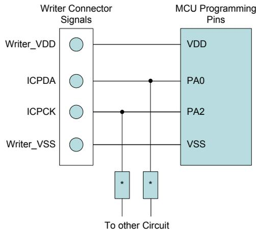
Note: \* may be resistor or capacitor. The resistance of \* must be greater than 1kΩ or the capacitance of \* must be less than 1nF.
