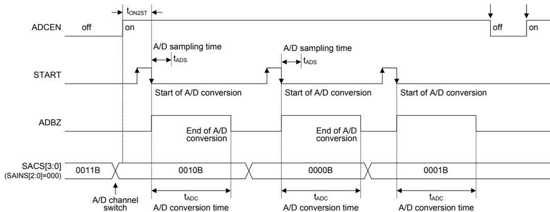
**Single A/D Conversion Timing – External Channel Input**
