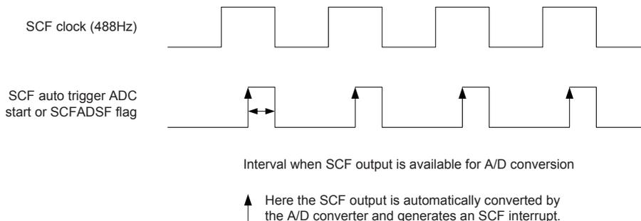
**SCF Signal Automatic A/D Conversion Timing**
