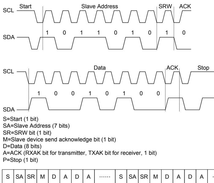
**I<sup>2</sup>C Communication Timing Diagram**
