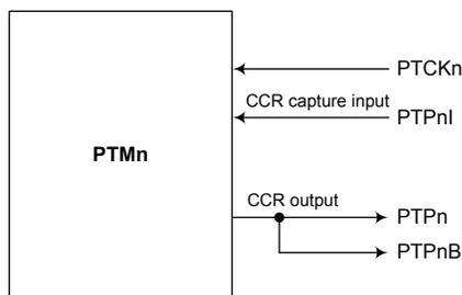
Note: Only the PTM0 has the inverted output pin PTP0B.
