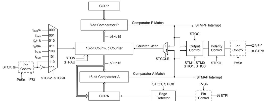
Note: The STPB is the inverted output of the STP.
