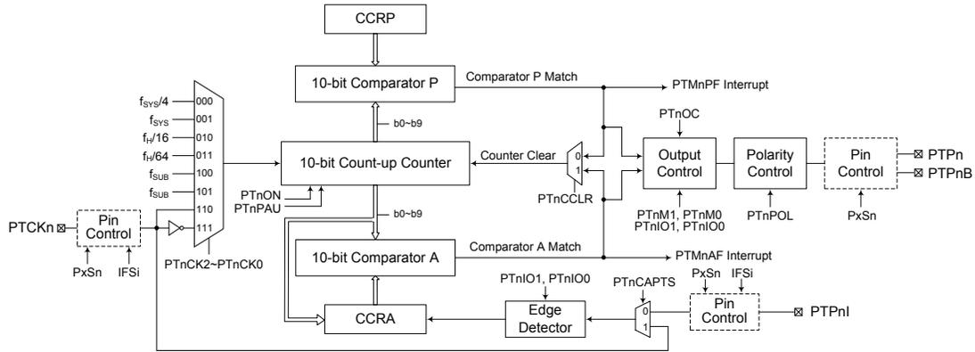
Note: The inverted output pin PTPnB and the external clock input source being selected using the IFSi register are only for the PTM0.
