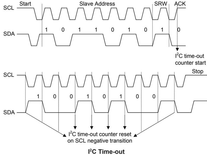
When an I<sup>2</sup>C time-out counter overflow occurs, the counter will stop and the SIMTOEN bit will be cleared to zero and the SIMTOF bit will be set high to indicate that a time-out condition has occurred. The time-out condition will also generate an interrupt which uses the I<sup>2</sup>C interrupt vector. When an I<sup>2</sup>C time-out occurs, the I<sup>2</sup>C internal circuitry will be reset and the registers will be reset into the following condition:
