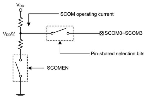
**Software Controlled LCD Driver Structure**
