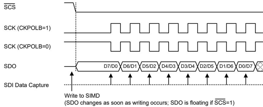
Note: For SPI slave mode, if SIMEN=1 and CSEN=0, SPI is always enabled and ignores the SCS level.
