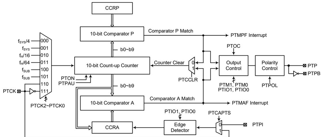
Note: The PTM external pins are pin-shared with other functions, so before using the PTM function the pin-shared function registers must be set properly to enable the PTM pin function.
