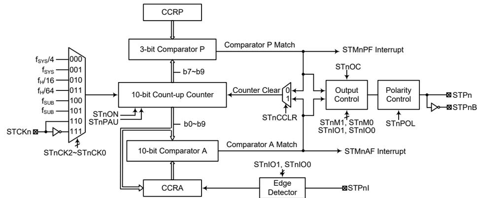
Note: The STMn external pins are pin-shared with other functions, so before using the STMn function, the pin-shared function registers must be set properly.
