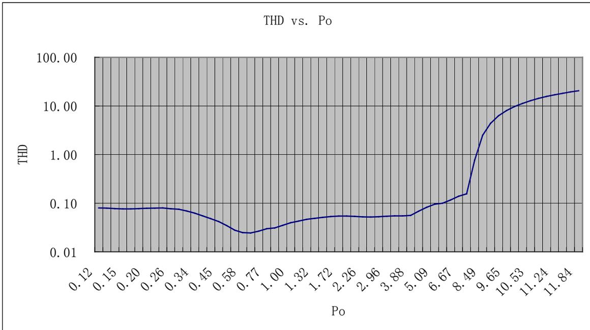
Figure 2 THND VS PO @ VCC=24V RL=8ohm
