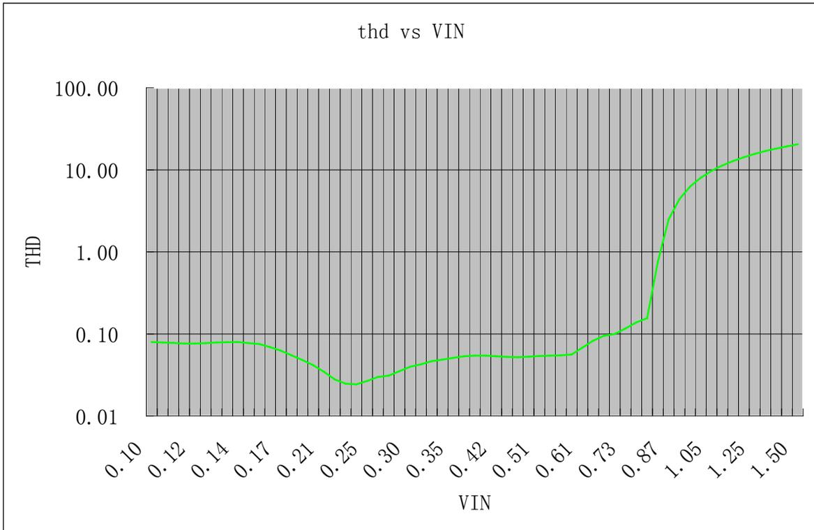
Figure 1 THND VS VIN @ VCC=24V RL=8ohm
