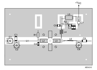
The circuit and the components are situated on one side of the P.T.F.E. fibre-glass board; the other side is unetched copper serving as a groundplane. Earth connections are made by using hollow rivets, fixing-screws and copper straps at the input and output and under the two emitters to provide a direct contact between the copper on the component side and the groundplane.
