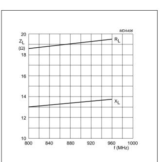
$V_{CE}$  = 12.5 V;  $P_L$  = 2 W; f = 800 - 960 MHz;  $T_{mb}$  = 25 °C; class-B operation; typical values.
