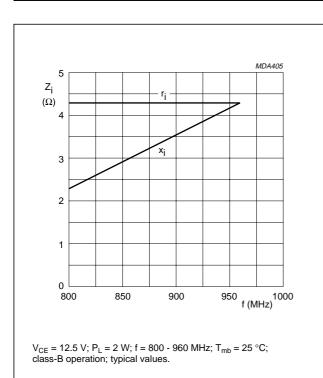
Fig.9 Input impedance (series components).
