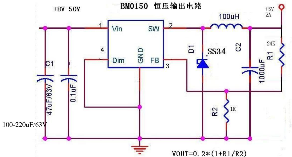
If the input voltage is high, the input capacitor C1, the larger the better, 100-2200uF
