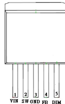
**BM0150HV can replace AP1509,AP1507,XL7005 without change PCB, the Vfb =0.2V, so need to modify one of the feedback resistor value.**
