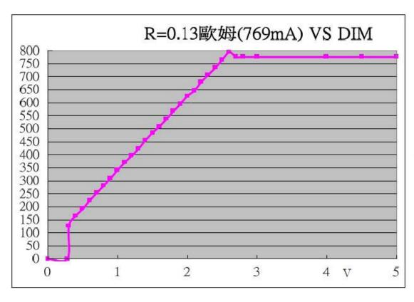
The BM0152HV allow dimming with a PWM signal at the DIM input. A logic level below 0.3V at DIM forces to turn off the LED and the logic level at DIM must be at least 2.5V to turn on the full LED current. The frequency of PWM dimming ranges from 100Hz to more than 20 kHz. The DC voltage is valid from 0.5V to 2.5V. When the dc voltage is higher than 2.5V, the output current keeps constant.
