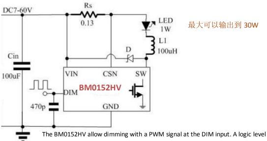
The BM0152HV allow dimming with a PWM signal at the DIM input. A logic level below 0.3V at DIM forces to turn off the LED and the logic level at DIM must be at least 2.5V to turn on the full LED current. The frequency of PWM dimming ranges from 100Hz to more than 20 kHz. The DC voltage is valid from 0.5V to 2.5V. When the dc voltage is higher than 2.5V, the output current keeps constant.
