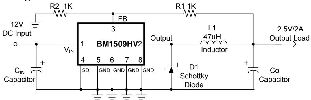
$$V_{OUT} = V_{FB} \times \left(1 + \frac{R1}{R2}\right)$$
