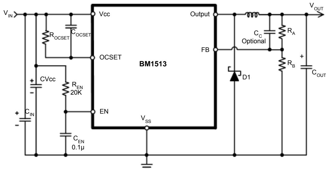
Note:  $V_{OUT} = V_{FB} \times (1 + R_A/R_B)$
