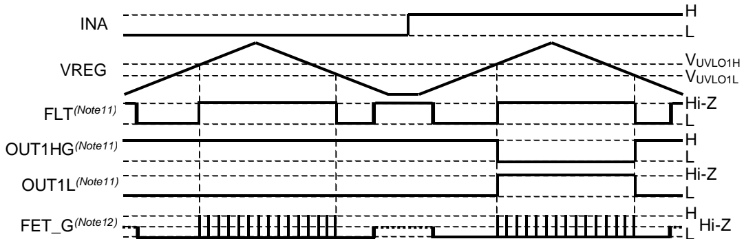
Figure 76. VREG UVLO Function Operation Timing Chart
