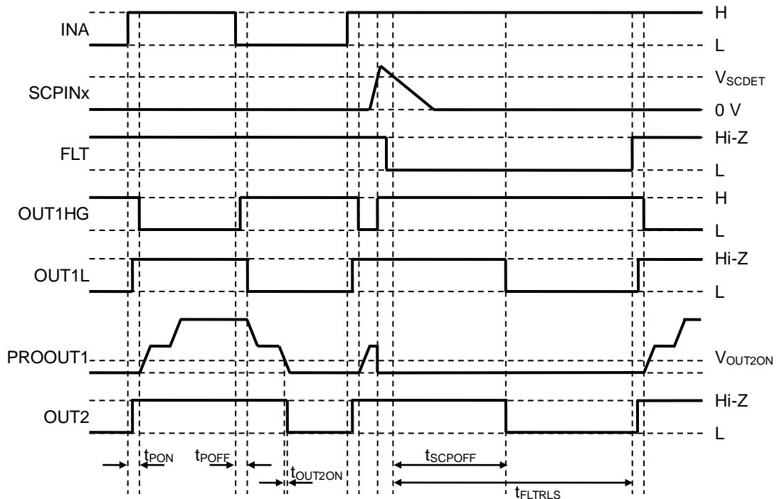
Figure 81. Timing Chart of Miller Clamp Function
