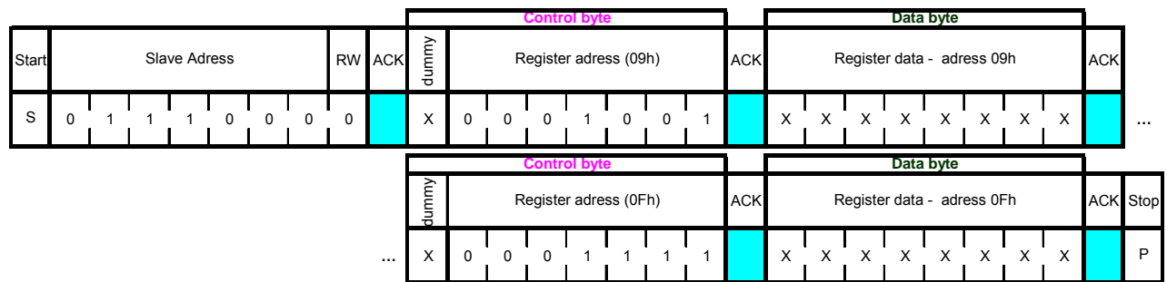
Figure 15: I 2 C multiple write protocol
