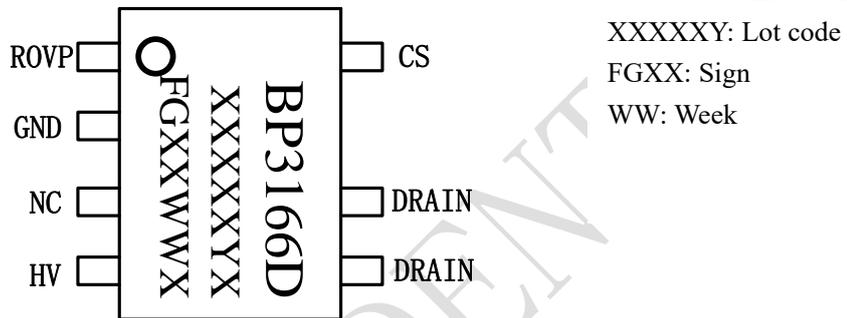
Figure 2. Pin configuration
