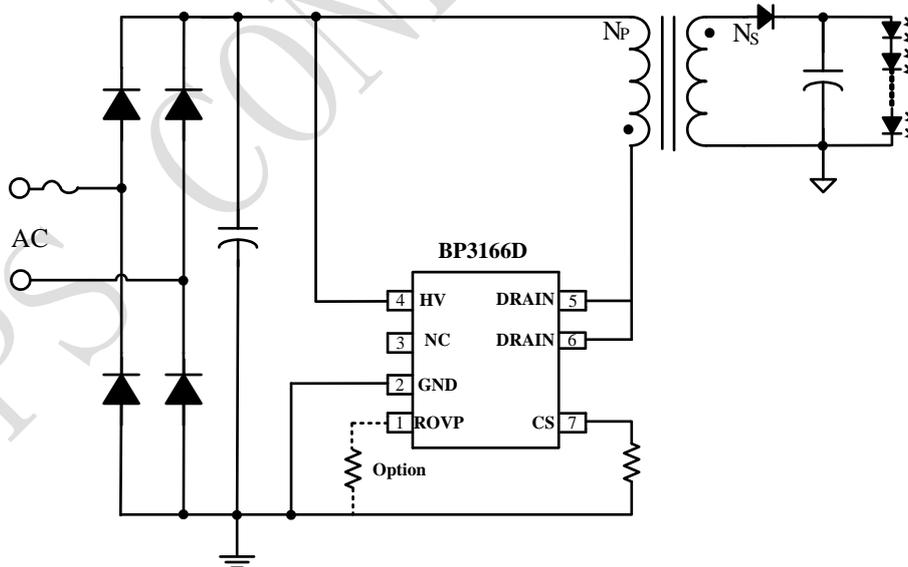
Figure 1. Typical application circuit for BP3166D
