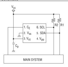
$C_p \dots 0.1 \mu F$ ...... 5k Ω R2 ......  $5k \Omega$
