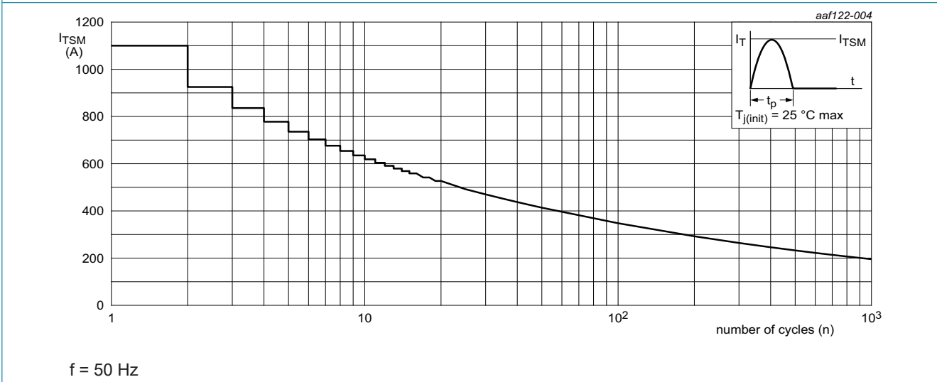
Fig. 4. Non-repetitive peak on-state current as a function of the number of sinusoidal current cycles; maximum values
