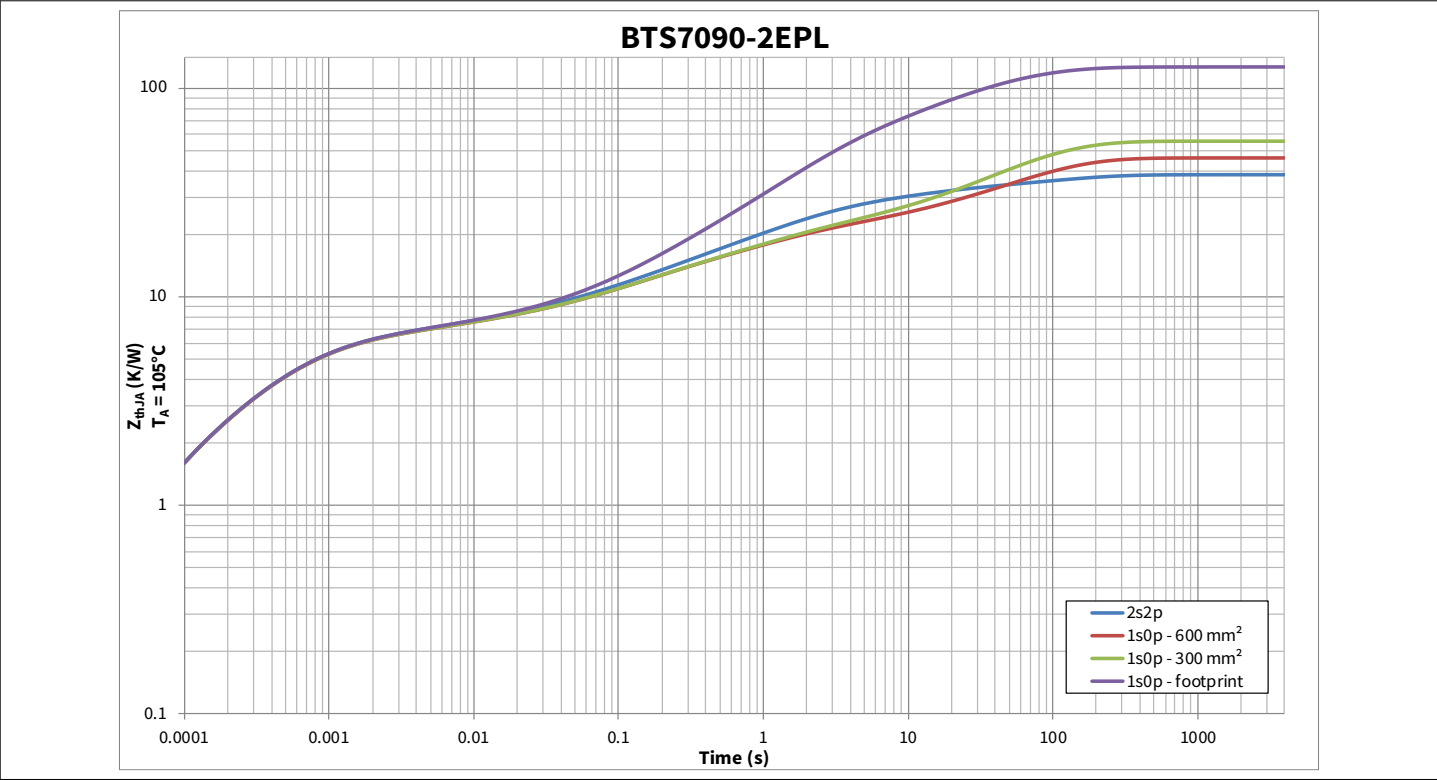
Figure 9 Typical thermal impedance. PCB setup according to PCB setup
