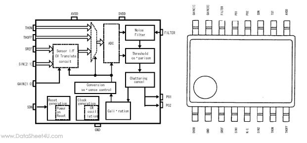
Sensor I/F CV Conversion Circuit:
