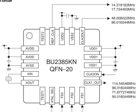
Note) BU2385KN is placed on the board normally. A decoupling capacitor  $(0.1\mu\text{F})$  needs to be placed between
