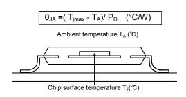
Figure 17. Thermal Resistance
