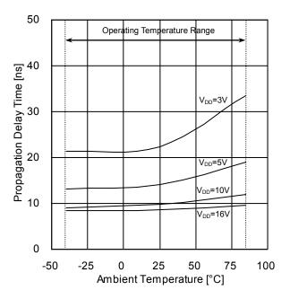
Figure 12. Propagation Delay Time  $t_{PHL}$  (IN $\rightarrow$ OUT) vs Ambient Temperature
