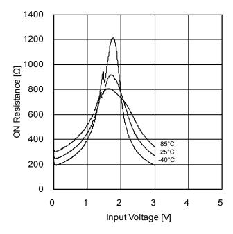
Figure 7. ON Resistance vs Input Voltage  $V_{\text{DD}}$ =3V
