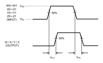
Figure 1. Propagation Delay Time (IN→OUT) (t<sub>PLH</sub>,t<sub>PHL</sub>)
