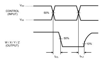
Figure 5. Propagation Delay Time (CONTROL $\rightarrow$ OUT) ( $t_{PZL},t_{PLZ}$ )
