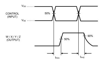
Figure 3. Propagation Delay Time (CONTROL→OUT) (t<sub>PLH</sub>,t<sub>PHL</sub>)
