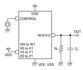
Figure 4. Test Circuit 2 (t<sub>PZH</sub>,t<sub>PHZ</sub>)
