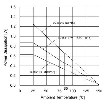
Figure 18. Derating Curve
