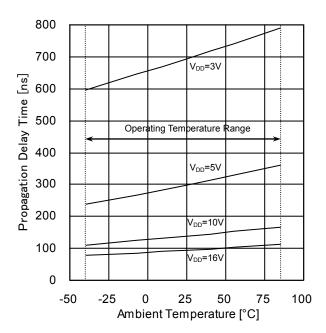
Figure 16. Propagation Delay Time  $t_{\text{PZL}}$  (CONTROL $\rightarrow$ OUT) vs Ambient Temperature
