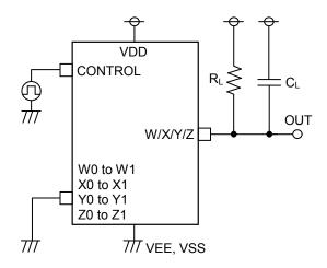
Figure 6. Test Circuit 3 ( $t_{PZL},t_{PLZ}$ )
