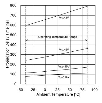
Figure 13. Propagation Delay Time  $t_{\text{PZH}}$  (CONTROL $\rightarrow$ OUT) vs Ambient Temperature
