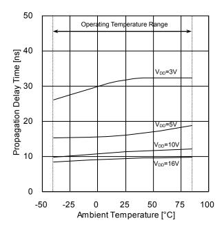
Figure 11. Propagation Delay Time t<sub>PLH</sub> (IN→OUT) vs Ambient Temperature
