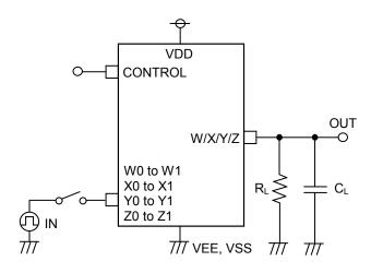
Figure 2. Test Circuit 1 (t<sub>PLH</sub>,t<sub>PHL</sub>)
