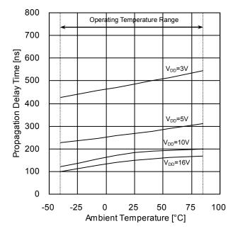
Figure 14. Propagation Delay Time  $t_{PHZ}$  (CONTROL $\rightarrow$ OUT) vs Ambient Temperature
