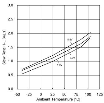
Figure 23. Slew Rate H-L vs Ambient Temperature
