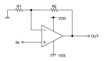
Figure 77. Non-inverting Amplifier Circuit
