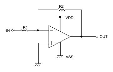
Figure 76. Inverting Amplifier Circuit
