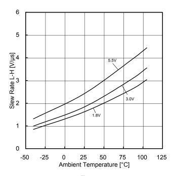
Figure 45. Slew Rate L-H vs Ambient Temperature
