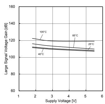
Figure 40. Large Signal Voltage Gain vs Supply Voltage
