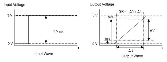
Figure 73. Slew Rate Input and Output Wave
