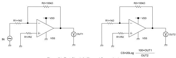
Figure 74. Test Circuit 3 (Channel Separation)
