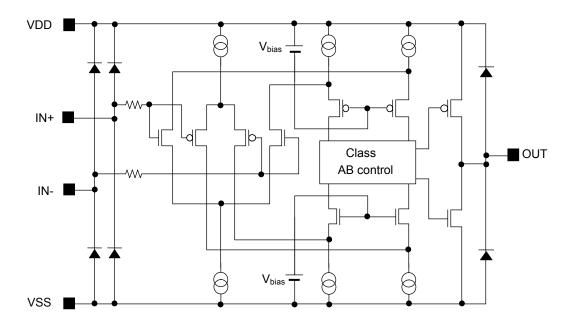
Figure 1. Simplified Schematic (1 channel only)
