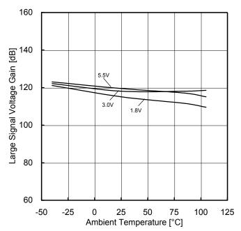
Figure 64. Large Signal Voltage Gain vs Ambient Temperature
