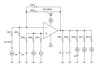
Figure 72. Test Circuit 2 (each channel)
