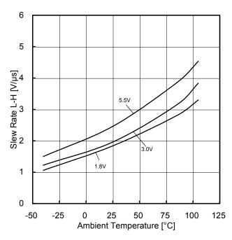
Figure 68. Slew Rate L-H vs Ambient Temperature
