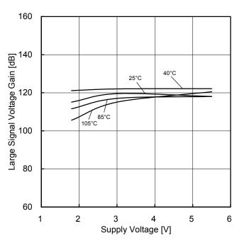
Figure 63. Large Signal Voltage Gain vs Supply Voltage
