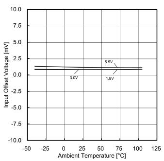
Figure 15. Input Offset Voltage vs Ambient Temperature  $(V_{ICM}=VDD, E_K=-VDD/2)$
