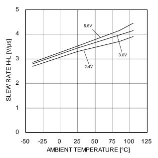
Figure 23. Slew Rate H-L – Ambient Temperature
