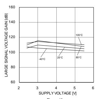
Figure 40. Large Signal Voltage Gain – Supply Voltage
