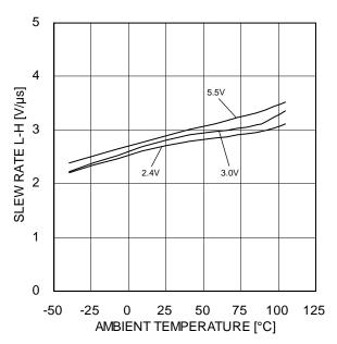
Figure 22. Slew Rate L-H – Ambient Temperature
