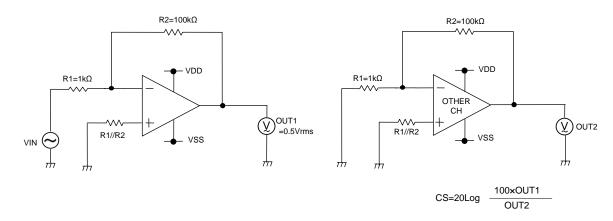
Figure 51. Test circuit 3 (Channel Separation)
