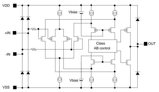
Figure 1. Simplified schematic (1 channel only)
