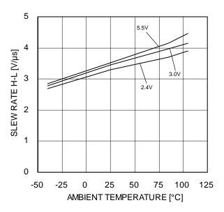
Figure 46. Slew Rate H-L – Ambient Temperature
