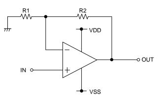
Figure 54. Non-inverting amplifier circuit
