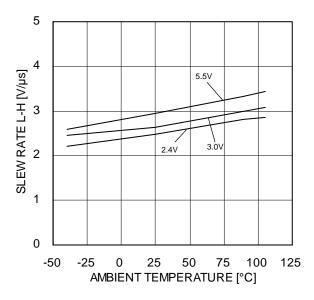
Figure 45. Slew Rate L-H – Ambient Temperature
