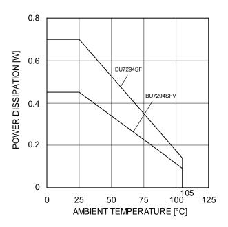
Figure 26. Derating curve
