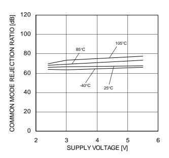
Figure 42. Common Mode Rejection Ratio – Supply Voltage
