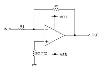
Figure 53. Inverting amplifier circuit
