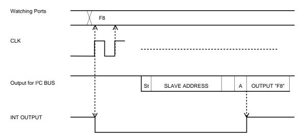
In the case that there is a change in detection ports once, and there are another changes before returning the ACK (as shown "A term"), then watching data is saved. And the output data in this case will be "AND" output of every bits of the watching data.
