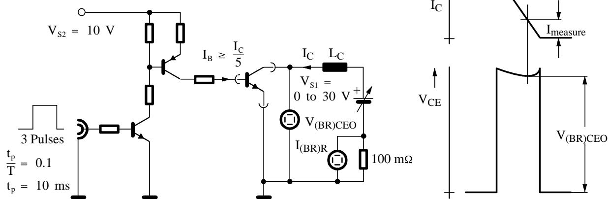
Figure 1. Test circuit for  $V_{(BR)CEO}$
