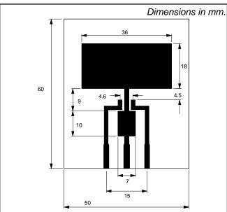
Fig.4. PCB for thermal resistance and power rating. PCB: FR4 epoxy glass (1.6 mm thick), copper laminate (35 μm thick).
