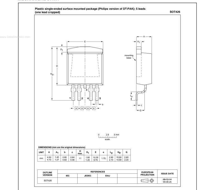
Fig.4. SOT426 surface mounting package<sup>1</sup>, centre pin connected to mounting base.
